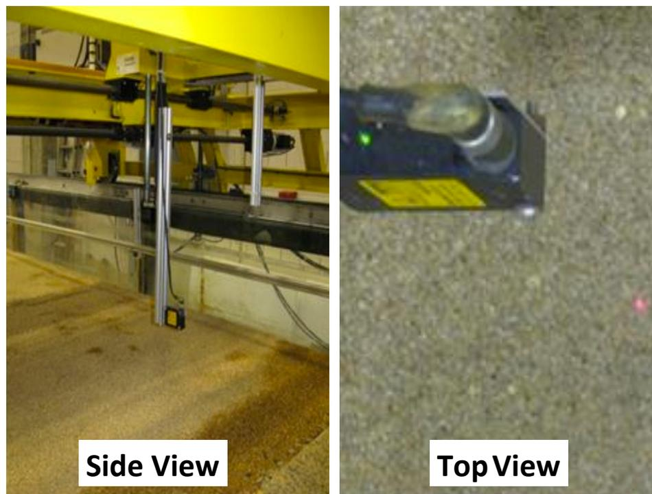
Figure 3.2 Point laser distance sensor
