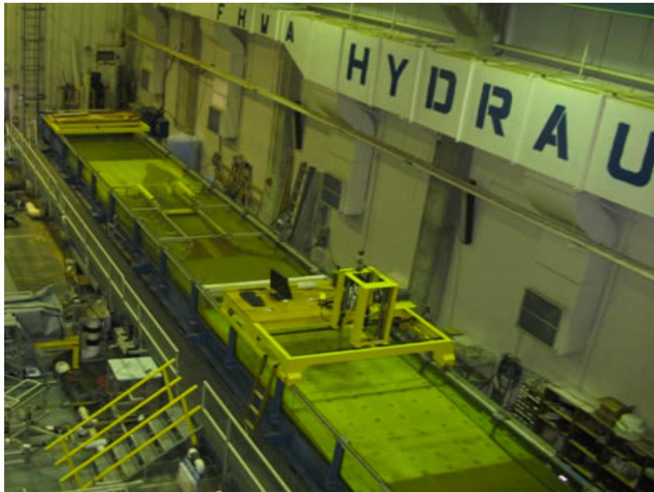
Figure 3.1 Tilting flume in FHWA hydraulic laboratory
