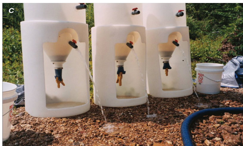
Figure 3. Sampling fine sediments from streams: A , diaphragm pump with hose and sieve attachment; B , sampling operation; C , settling tanks.
