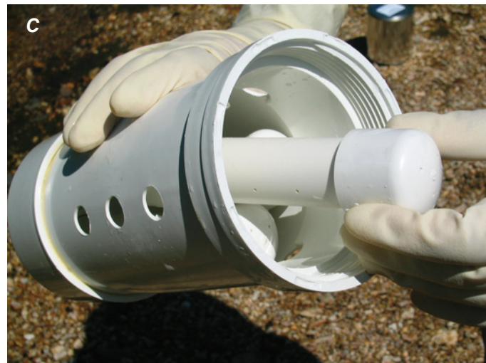
Figure 4. In-stream, passive sampling apparatus: A , "peeper" (pore-water diffusion sampler); B , opened housing containing stabilized liquid membrane device (passive integrative water sampler); C , outer canister containing three sampler housings.
