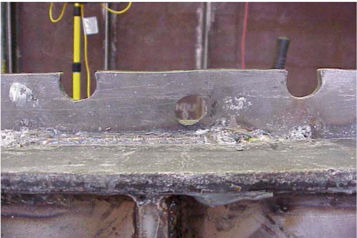
Figure 3-120: Close up of Perforated Plate after Test
