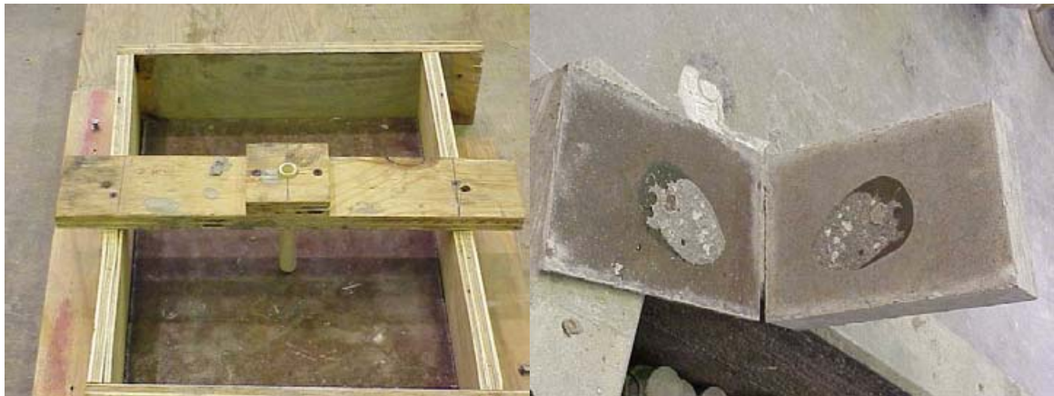
Figure 3-17: Form with injection tube in place
