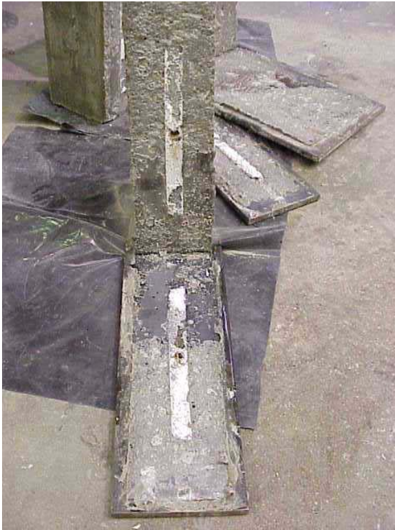
Figure 3-27: Specimen Dismantled showing spread of epoxy
