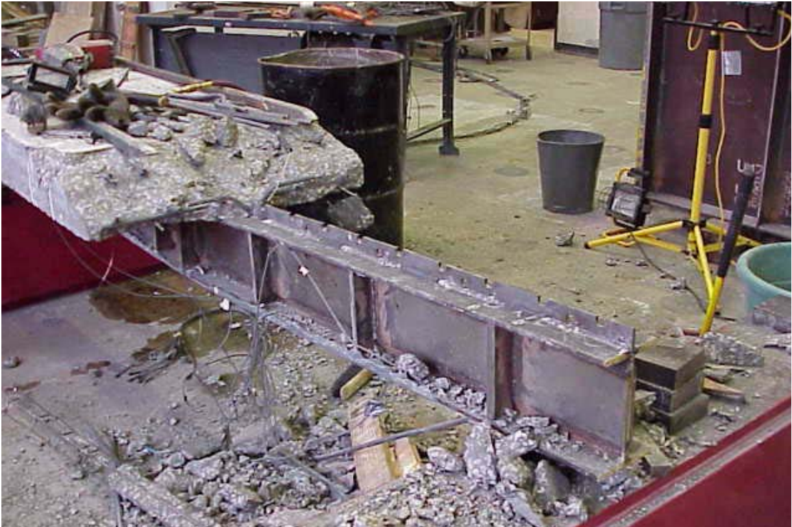
Figure 3-119: Specimen with Concrete Removed
