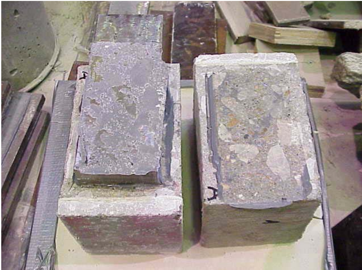
Figure 3-66: Close-up of failure cut specimen
