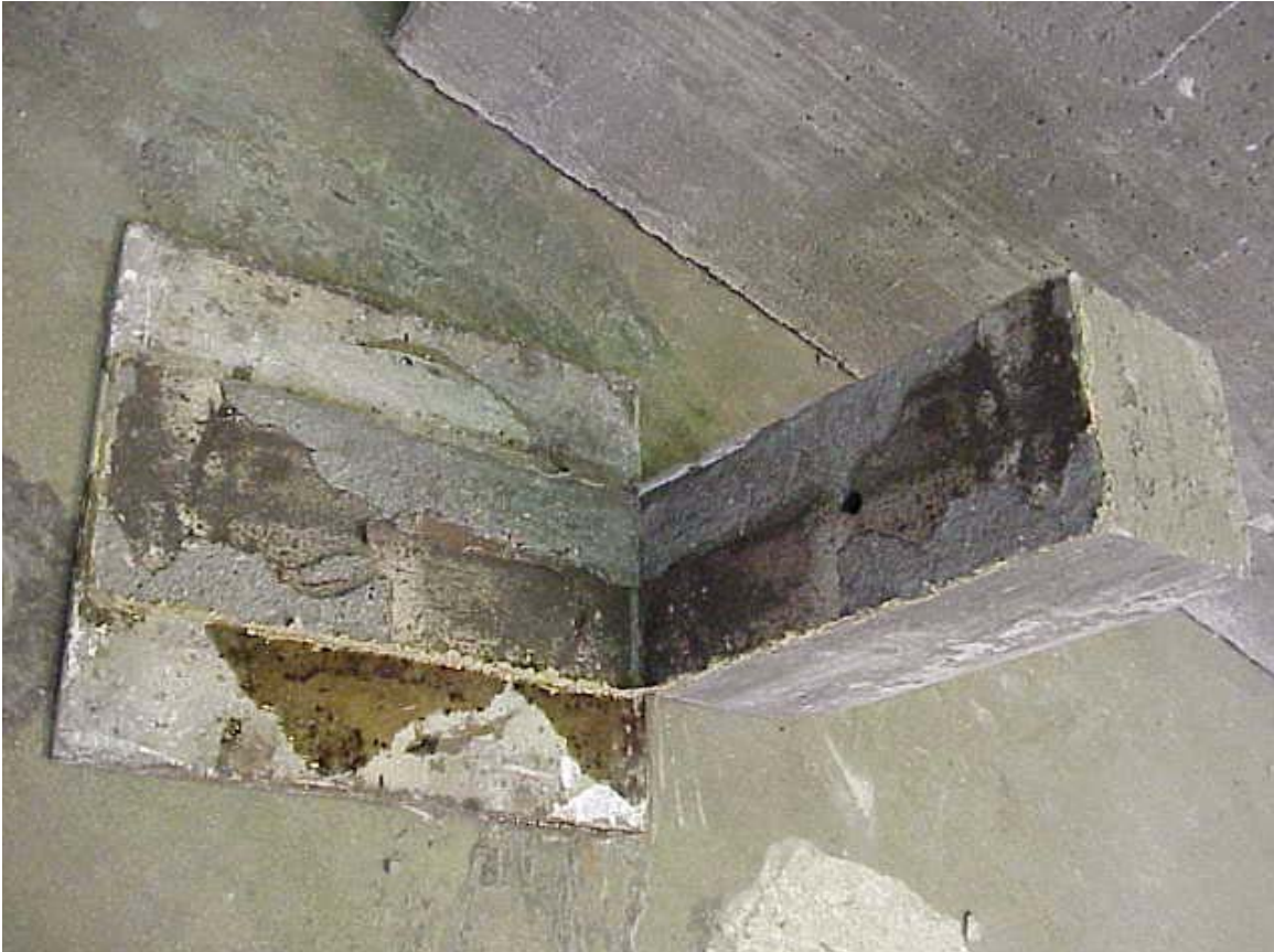
Figure 3-22: Specimen showing spread of epoxy
