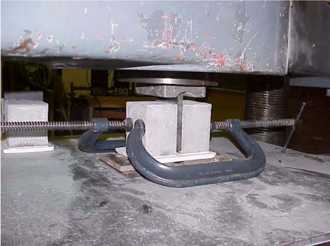
Figure 3-58: Test Setup with C-Clamps
