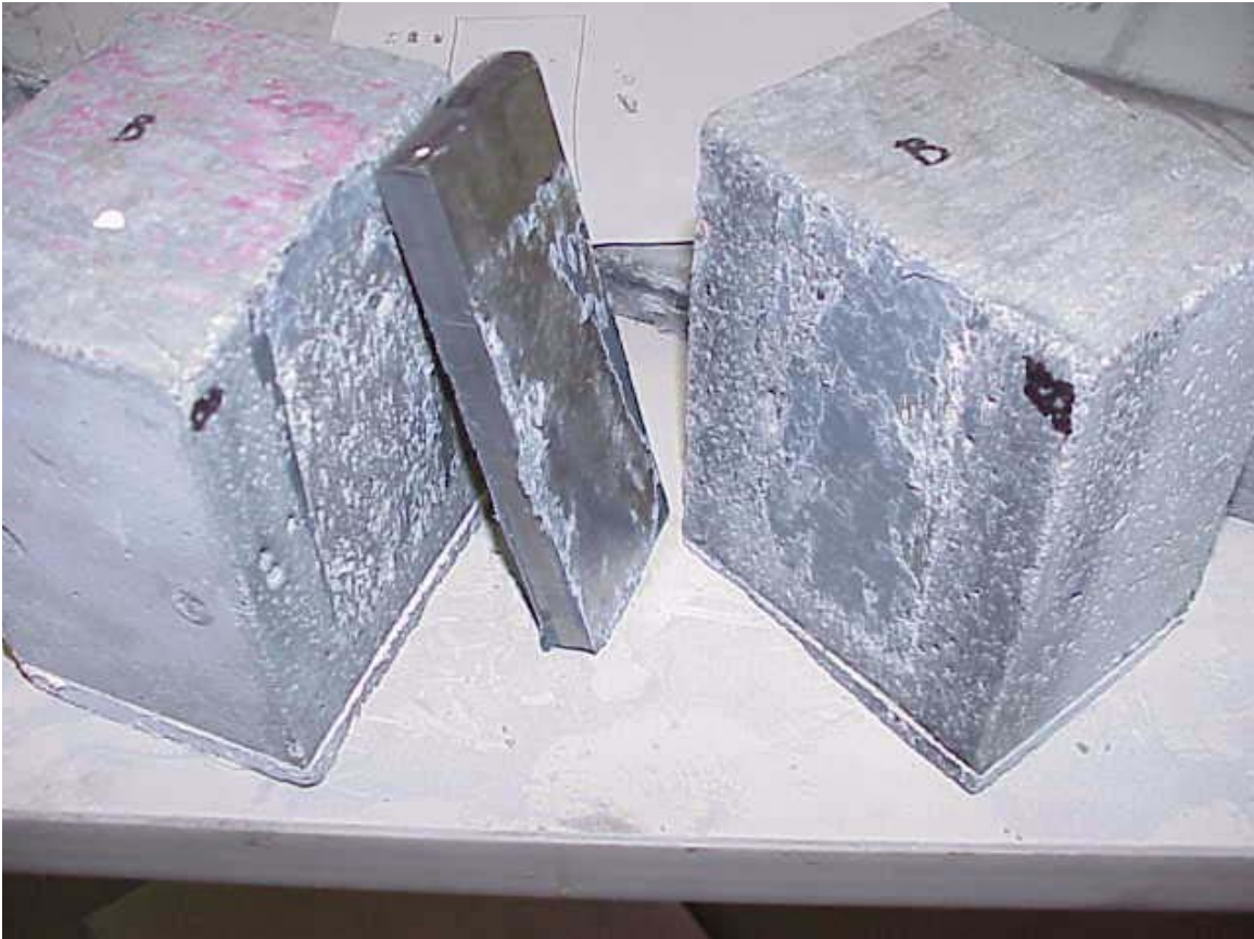
Figure 3-65: Close-up of failure wire prepped specimen
