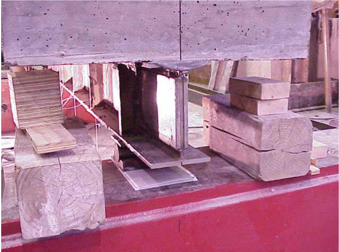
Figure 3-70: Close-up of Epoxy Beam Specimen End Support
