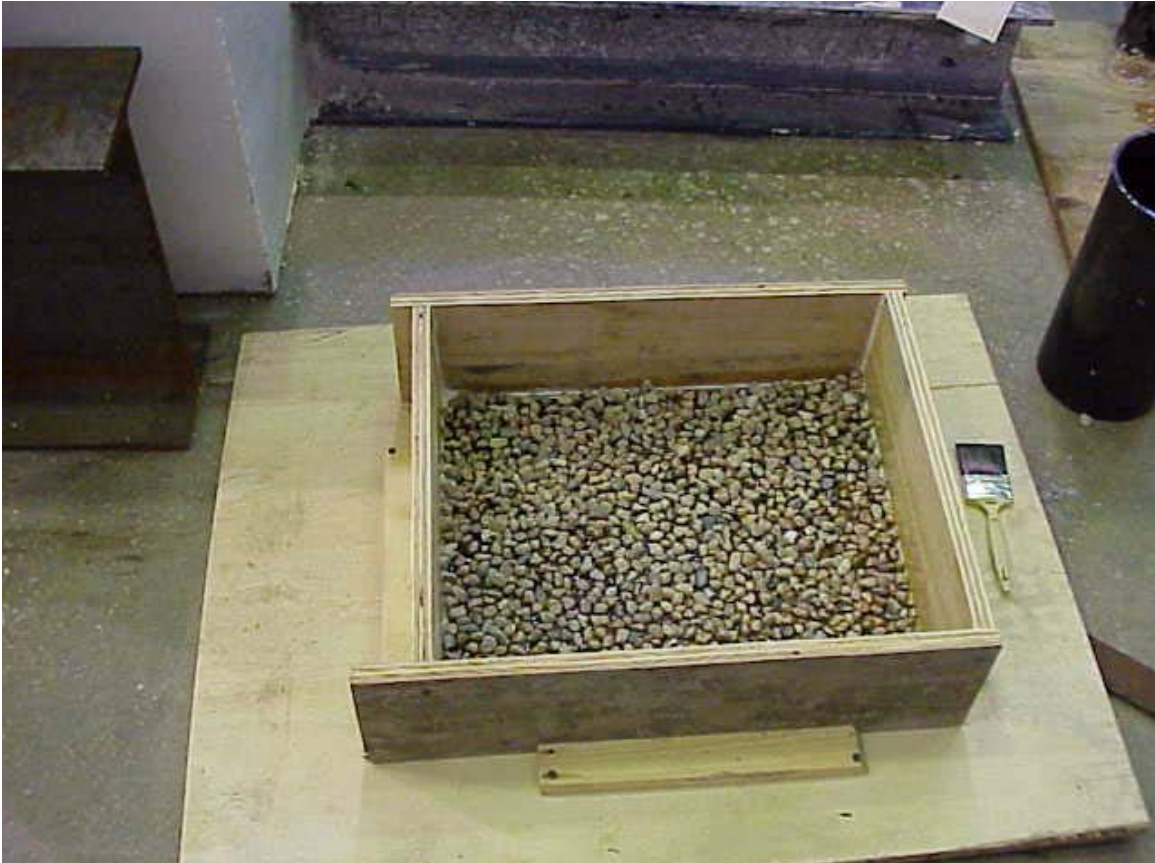
Figure 3-109: Pebbles bonded to steel
