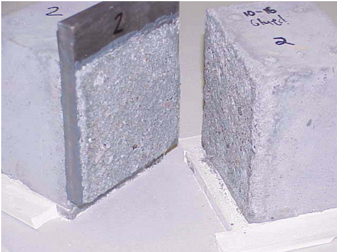
Figure 3-61: Close-up of failure second specimen
