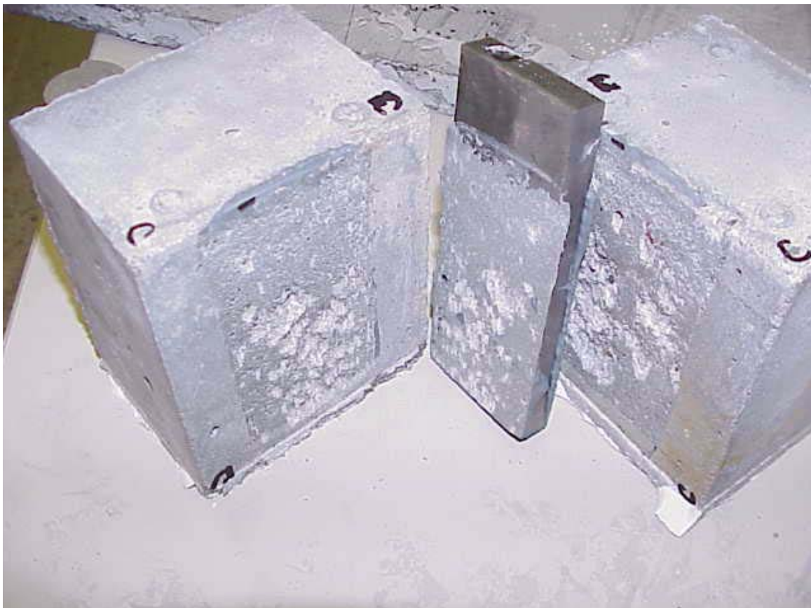
Figure 3-64: Close-up of failure control specimen
