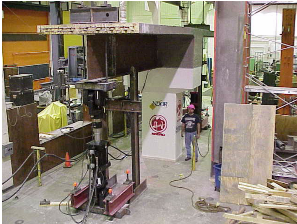
Figure 6-35: Fatigue Loading System (Alternate View)
