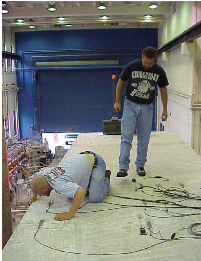
Figure 7-7: Deck Crack Mapping
