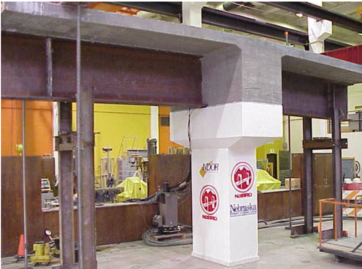
Figure 6-36: Ultimate Capacity Loading System (Side View)
