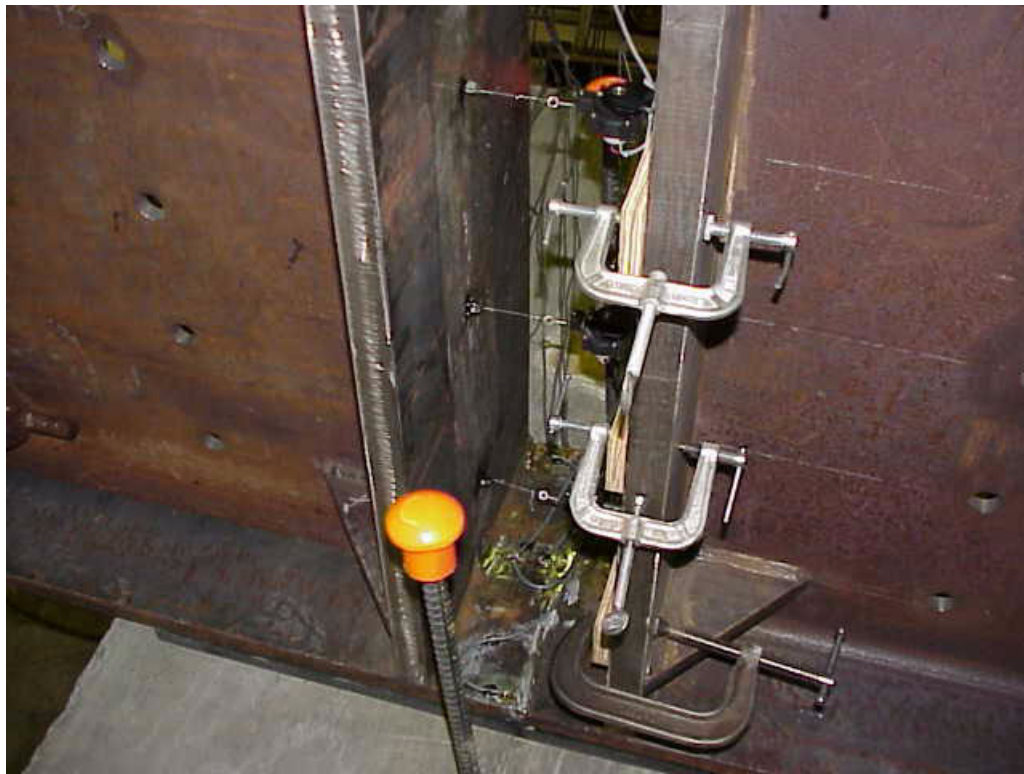
Figure 6-33: Dead Load Potentiometers (Alternate View)
