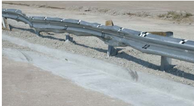
Figure 111. System Damage, Test NPG-5
