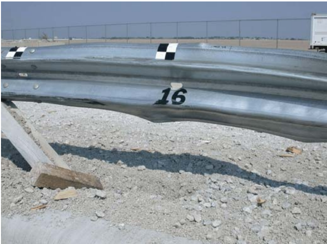
Figure 113. System Damage, Test NPG-5
