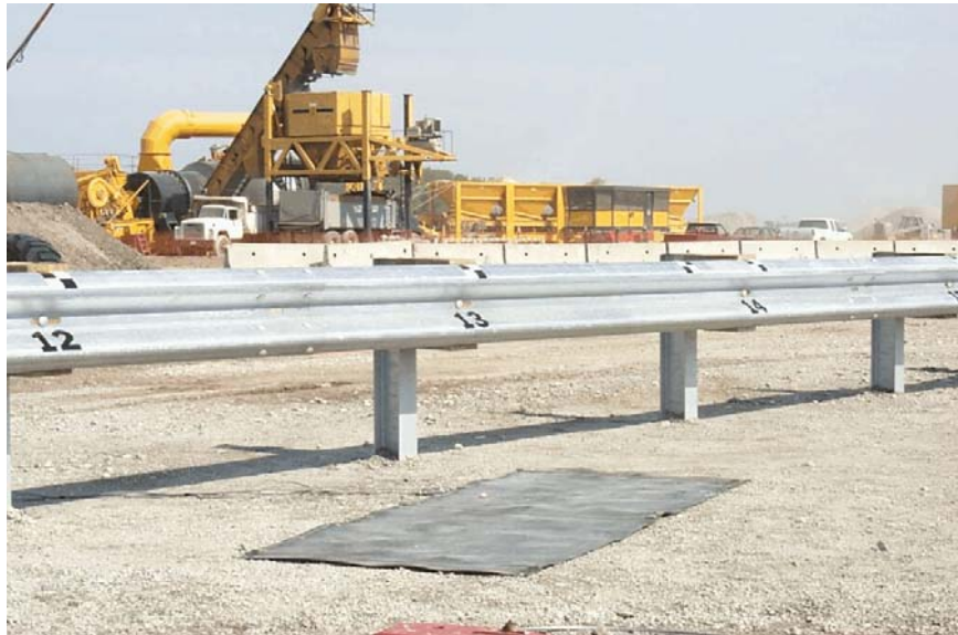
Figure 35. Midwest Guardrail System Maximum Height Tolerance
