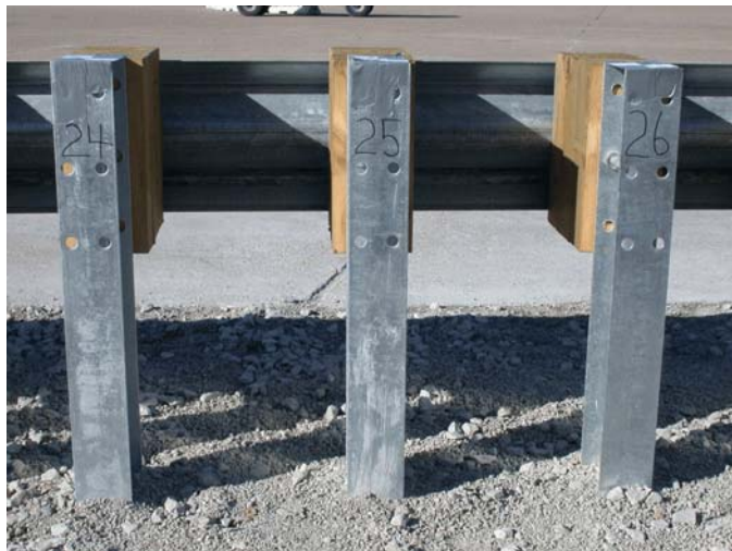
Figure 122. Reduced Post Spacing Midwest Guardrail System
