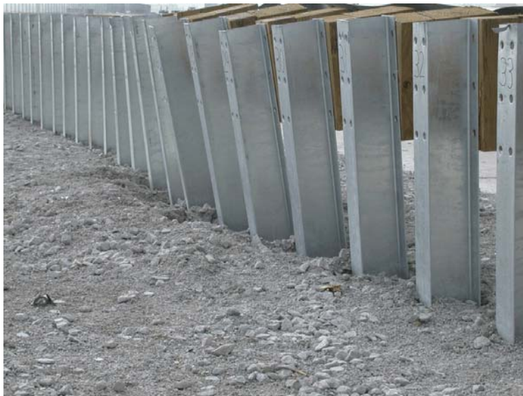
Figure 132. System Damage, Test NPG-6
