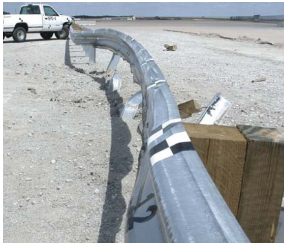
Figure 94. System Damage, Test NPG-4
