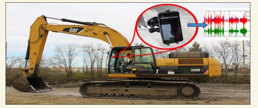
After data collection was completed, it was analyzed in the lab. The video data was timestamped at one second intervals of the activity that the construction equipment was performing. The time-stamped data was then fed into a machine learning algorithm and data classifier program known as Weka.
