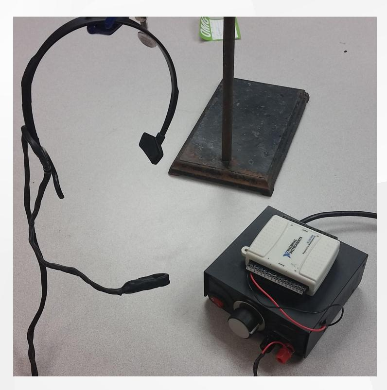
Figure 1. Hotwire anemometer and power source
