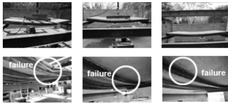
Photographic record of Type I and Type II Specimen Failures
