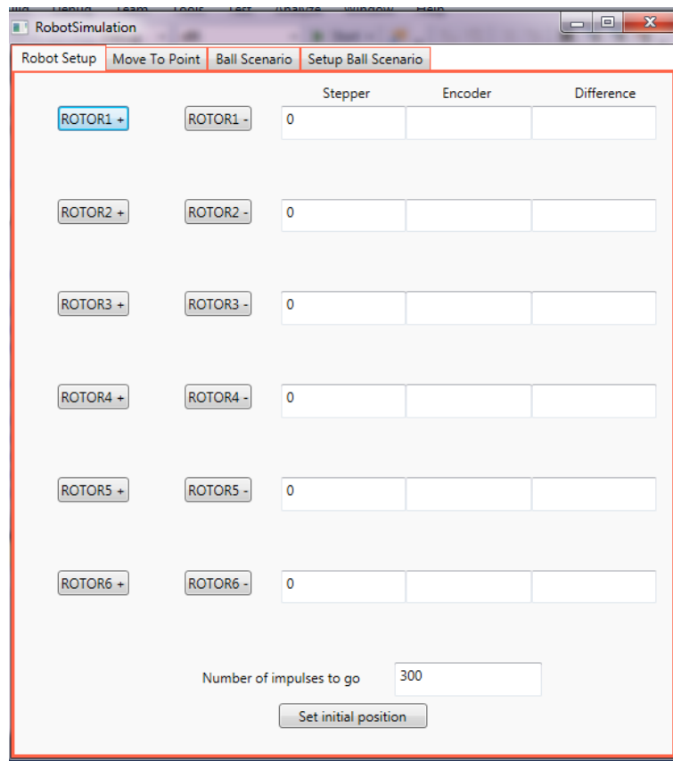
Figure 4.6: User interface of the tab for setting the initial position of the robotic arm.
