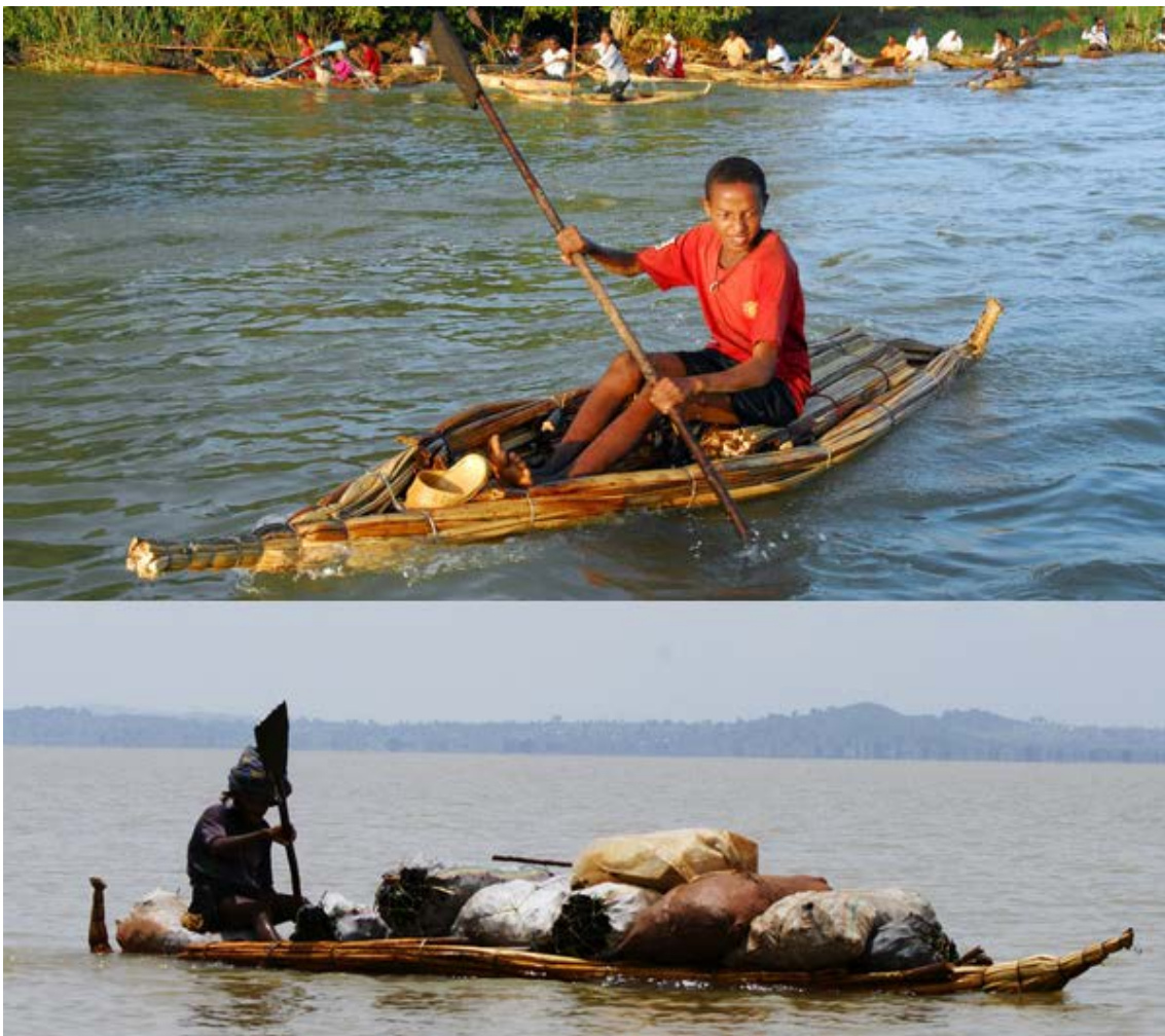
Figure 29: Reed boat: very simple kayak- like shaped Tankawa papyrus boat paddled by two bladed paddle on Lake Tana, Ethiopia (Photography top: Brian J. McMorrow [On line] Available at: < http://www.pbase.com/image/108955080 >) (Photography bottom: "Djib" by Flickr [On line] Available at: < https://www.flickr.com/photos/99631178\spacefactor\@mN00/2645782736 > [29. May 2015]).
