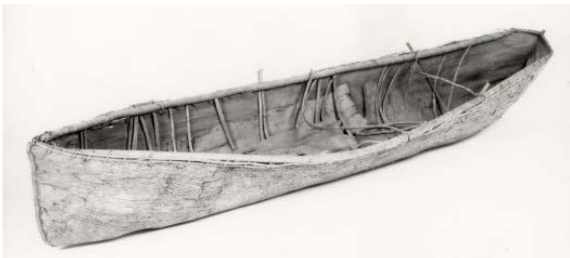
Figure 15: Bark boat: Type of Australian Sticked bark boat made from birch bark from South East Australia (Photography: Australian National Maritime Museum [On line] Available at: < http://australianmuseum.net.au/blogpost/science/tentative-chronology-of-indigenous-canoes-of-eastern-australia > [29. May 2015])
