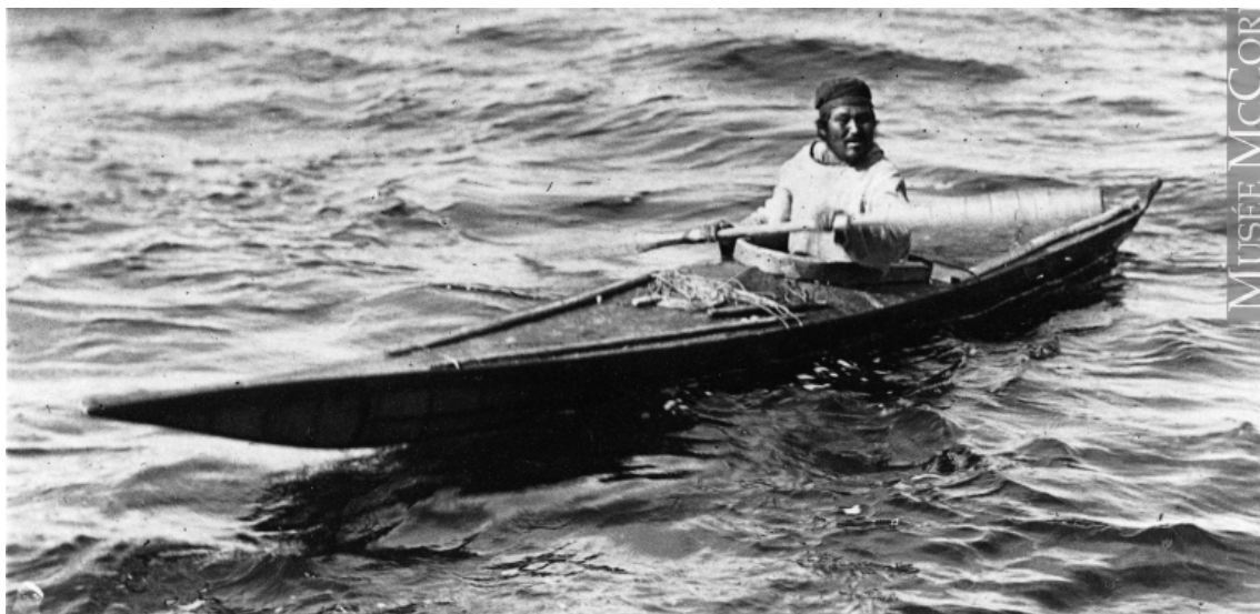
Figure 11: Skin boat: Kayak mostly made by seal skin and whalebone skeleton (Photography: Samuel Herbert Coward; McCord Museum, Montreal, Quebec [On line] Available at: < http://www.mccord-museum.qc.ca/scripts/large.php?Lang=1&accessnumber=MP-1976.24.64&idImage=192484 > [29. May 2015])
