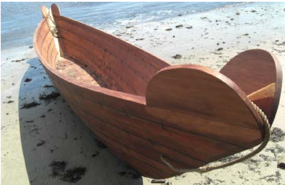
Figure 50: Plank boat: Typical Indian plank boat ' Elye'wun ' of Chumash people from south California. Boat is "V" formed chine (Photography: ©Chumash Maritime Association [On line] Available at: < http://www.chumashmaritime.org/Home.html > [29. May 2015]).
