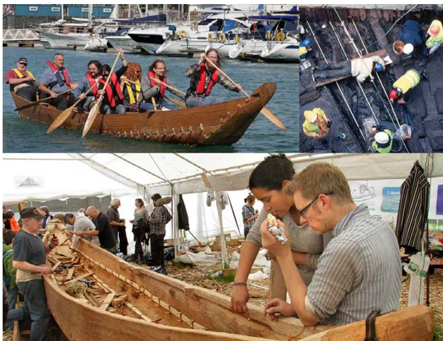
Figure 46: Plank boat: Dover boat was constructed of oak planks, stitched together with yew withies and also fixed together with wooden wedges ( Top left: Paddling a half scale replica, top right: Excavation in 1992 and bottom: Replica reconstructing 2013 [On line] Available at: < http://www.canterburytrust.co.uk/trust-blog/ > [29. May 2015]).
