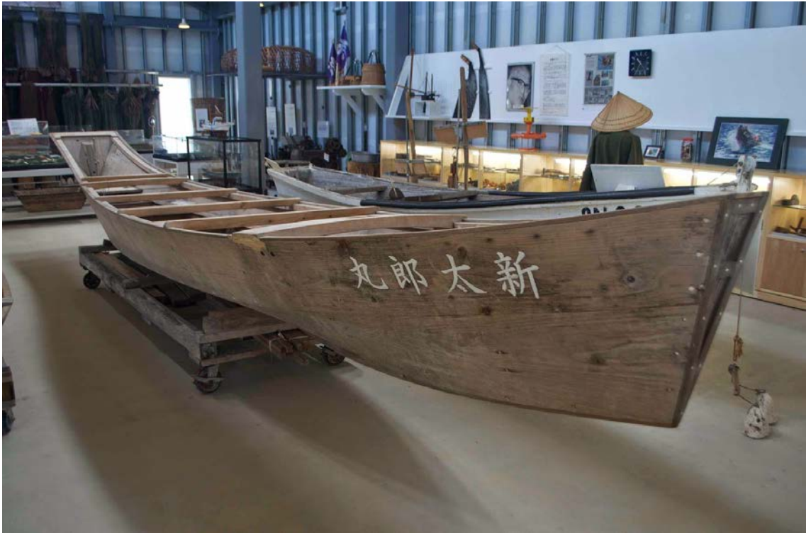
Figure 49: Plank boat: Typical plank boat sabani from fishing port Itoman in Okinawa. Boat is "V" formed chine and fastened with hardwood butterfly keys huundu (Photography: Douglas Brooks [On line] Available at: < http://blog.douglasbrooksboatbuilding.com/2014/07/okinawa.html > [29. May 2015]).
