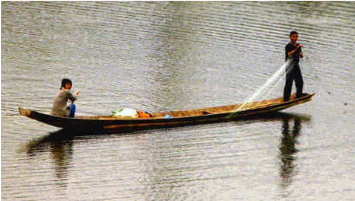
Figure 47: Plank boat: Typical Three- plank boat sampan from Mekong river in Laos. Boat is flat bottomed, with shovel ends, flaring sides, and quite long for their width. It is joined and stitched with rattan or bamboo strips, which in later times were replaced by bamboo nails or iron nails. A further improvement was the use of tenoning. (Photography: Ken Preston [On line] Available at: < http://www.boatsandrice.com/Lmekong.html > [29. May 2015]).
