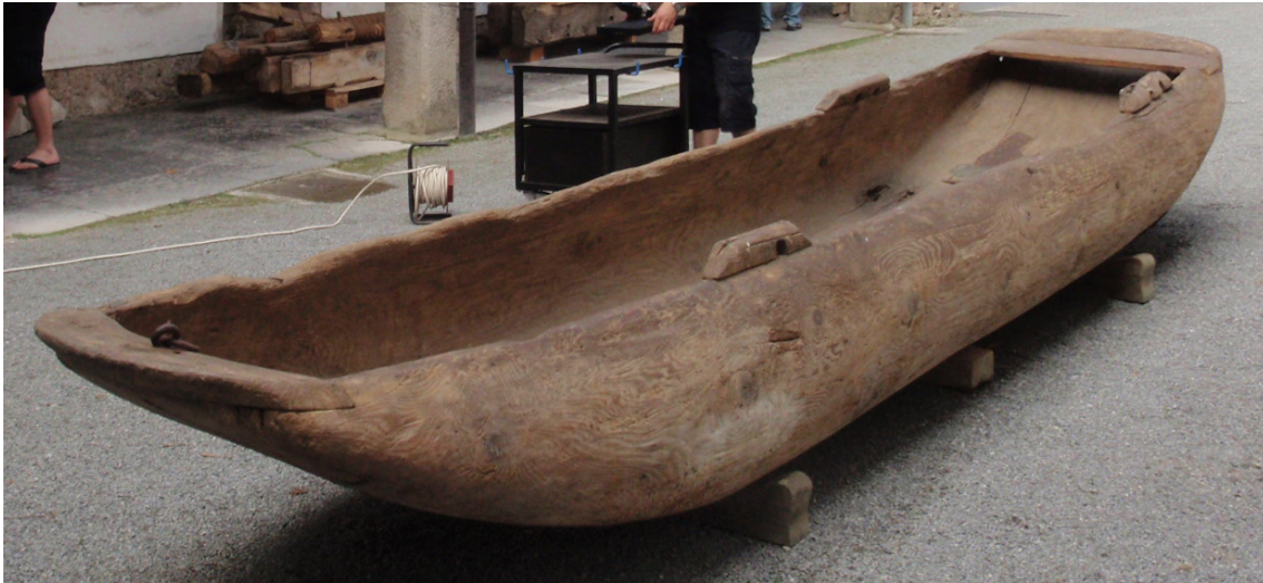
Figure 21: Logboat: Special autochthonous construction of multi- extended logboat caled drevak which mean tree- boat, isolated in Notranjska region, Slovenia, perhaps with the roots in Roman period. It is made from fir with two part of logboat as chine-girders with one or two inserted bottom planks. Exposed in Technical Museum of Slovenia, Bistra (Photography: Miran Erič).
