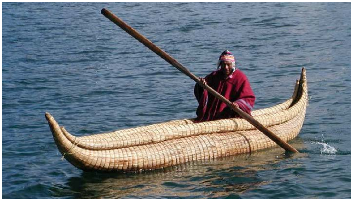
Figure 32: Reed boat: Lake Titicaca between Peru and Bolivia is one of the most known areas in the world where reed boats are still part of the everyday lives of the locals. The boats are all named balsa and vary in size from small to as large as 30m long. Typical totora bullrush small canoe-like boat from the Lake. (Photography: Andre Engels [On line] Available at: < https://en.wikipedia.org/wiki/Reed_boat > [29. May 2015]).
