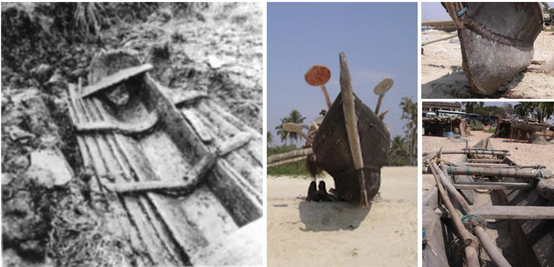
Figure 22: Logboat: Left Type of typical European 13 rd century extended logboat with side planks coupled with the ribs from Kentmere, Cumbria discovered by David G. Wilson. (Photography: David Wilson; Seán McGrail, Ancient Boats in North-West Europe. The Archaeology of Water Transport to AD 1500 , Longman AS 1998, p. 75, figure 6.15). Right Typical extended modern logboat use in Goa, India with high exposed constructional solution. Today extended logboats are often in combination with outriggers logboats specially for using on seas (Photography: Paul Wilson, Archive of Indigenous boat blog site of Bob Holtzman [On line] Available at: < http://counter-agency24.rssing.com/chan-12927004/all_p1.html > [29. May 2015]).
