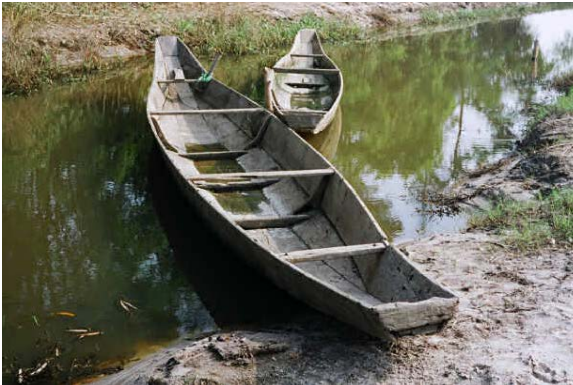
Figure 48: Plank boat: Typical Vietnamese Five- plank boat from Central coast and Ron river. Boat is flat bottomed, with shovel ends, flaring sides, and quite long for their width. (Photography: Ken Preston [On line] Available at: < http://www.boatsandrice.com/cVN.html > [29. May 2015]).
