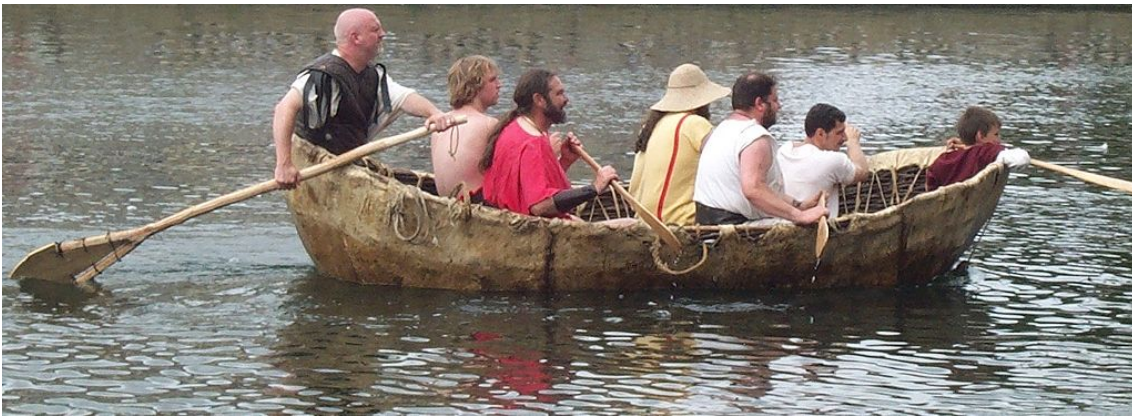
Figure 6: Skin boat: A reconstruction of a first century AD British Curragh (a big coracle), made of wicker work and covered with 3 cow hides. It is capable of carrying 10 people. It was being paddled on the River Great Ouse at the 2008 Bedford River Festival. (Photography: Simon Speed [On line] Available at: < http://en.wikipedia.org/wiki/Currach#/media/File:FloatingCurraghBedford.JPG > [29. May 2015])
