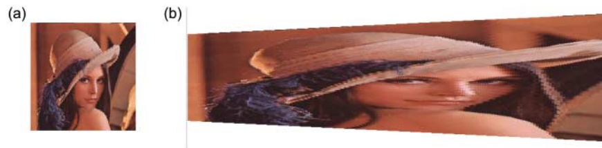
Figure 5. (a) Undistorted predetermined image. (b) Anamorphic projected image corresponding to viewer position (10, 0, 2). To see the anamorphic image undeformed, look at it from the right side with the face just above the plane of the paper.
