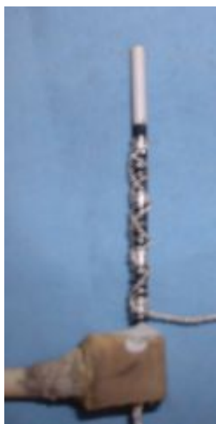
Figure 18: "SOFC" SOFC tube
