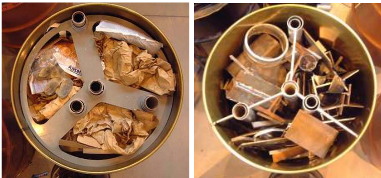
Figure 54: Axial view of two 205l drums filled with artificial soft and hard matrices.
