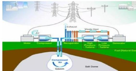
Figure 3: Compressed Air Energy Storage in Salt Caverns
