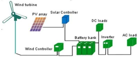
Figure 1: Solar-Wind-Battery Hybrid System
