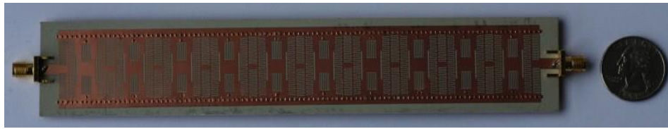
Figure 3.19 (a) Equivalent circuit of one ECRLH unit cell; (b) photograph of the fabricated LWA based on the ECRLH structure [36].
