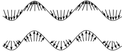
Fig. 2. Particle motion of the antisymmetric Lamb wave mode [8].
