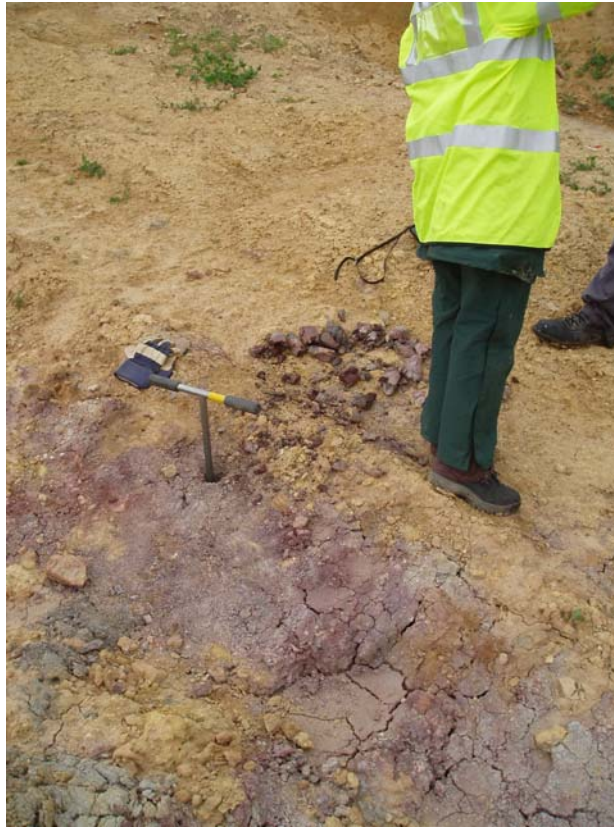
Figure 8 (Locality 1). Weathered Carboniferous mudstone of the Lower Coal Measures Formation exposed in the bottom of the excavation and proved by hand auger to a depth of 1m.
