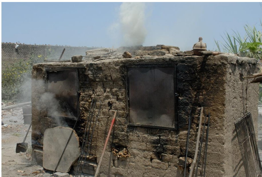
Picture 4: Kiln where Chulucanas type pottery is fired with mango leaves
