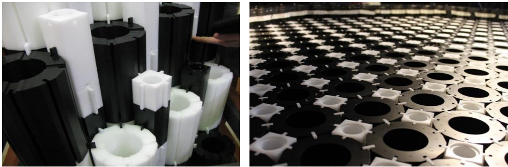
Fig. 5 - Quarter scale Acetal components in the MLA rig (left: columns, right: top layer)
