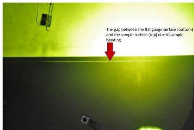
Figure 5: The Gap between the Sample and the Gauge Surface
