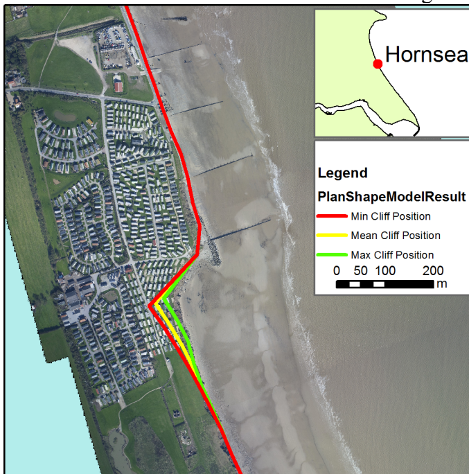
Figure 16 Representation of the modelled probabilistic behaviour of the cliff at the southern end of the Hornsea defences throughout a ten-year period
