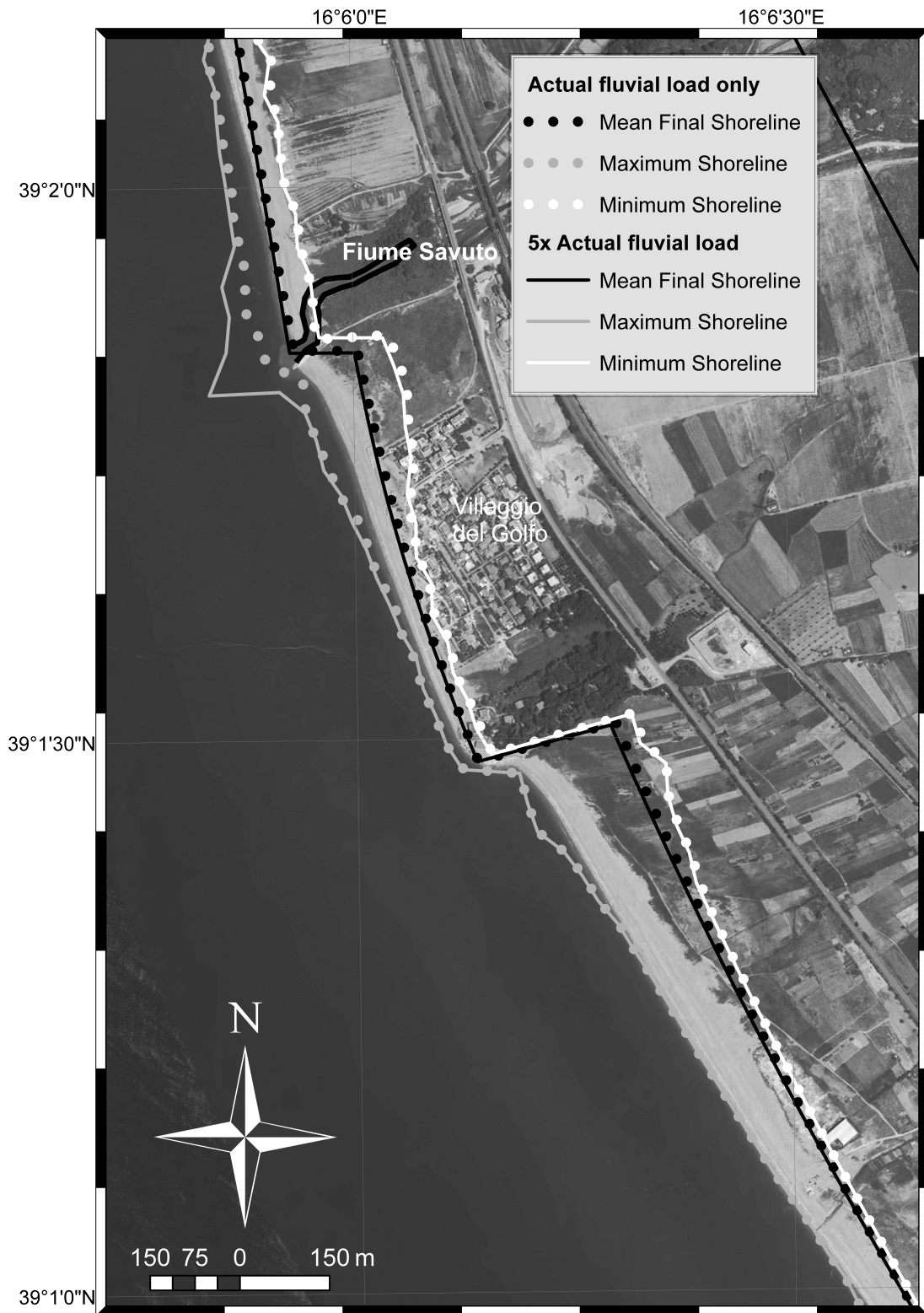
Figure 10 Comparison of probabilistic simulations of future shoreline evolution given (a) present-day fluvial loading (dotted) and five-times present-day fluvial loading (solid), without beach nourishment practice, (b) examining the influence of timing of beach nourishment, and (c) examining the influence of nourishment volume
