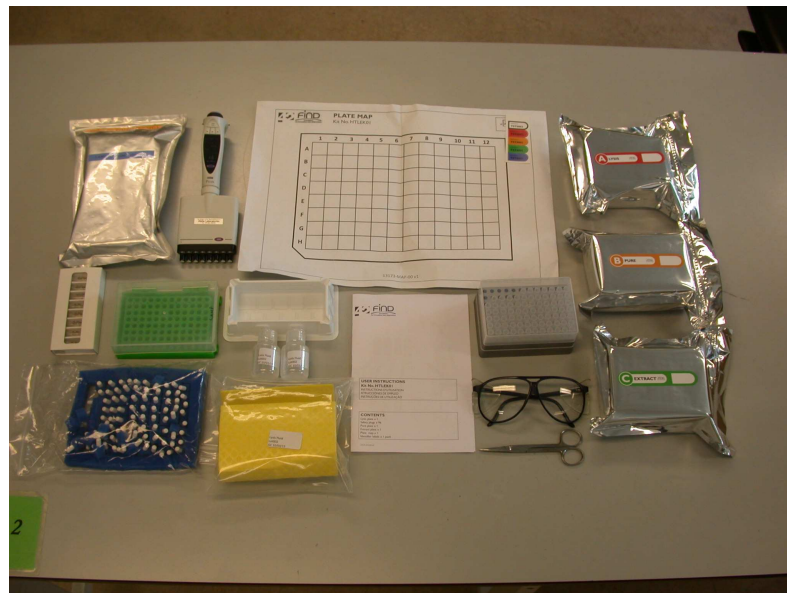
Fig 1. Layout of the contents of the high throughput sample processing kit on the bench. The contents of the sample processing kit which includes a LYSIS plate, PURE plate, EXTRACT plate, sample record sheet, lysis fluid, individual foam plugs and instruction manual.
