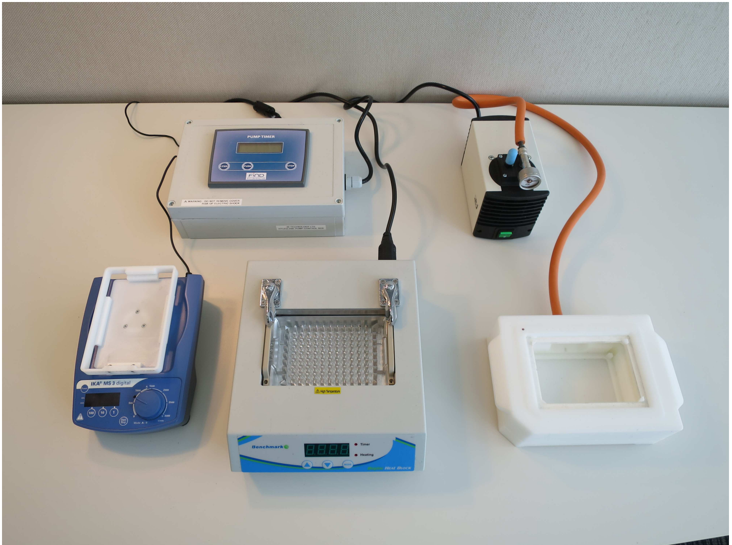
Fig 2. Layout of the high throughput set-up on the bench. The layout of the high throughput set-up which includes a shaker, hot block, vacuum manifold and pressure gauge.
