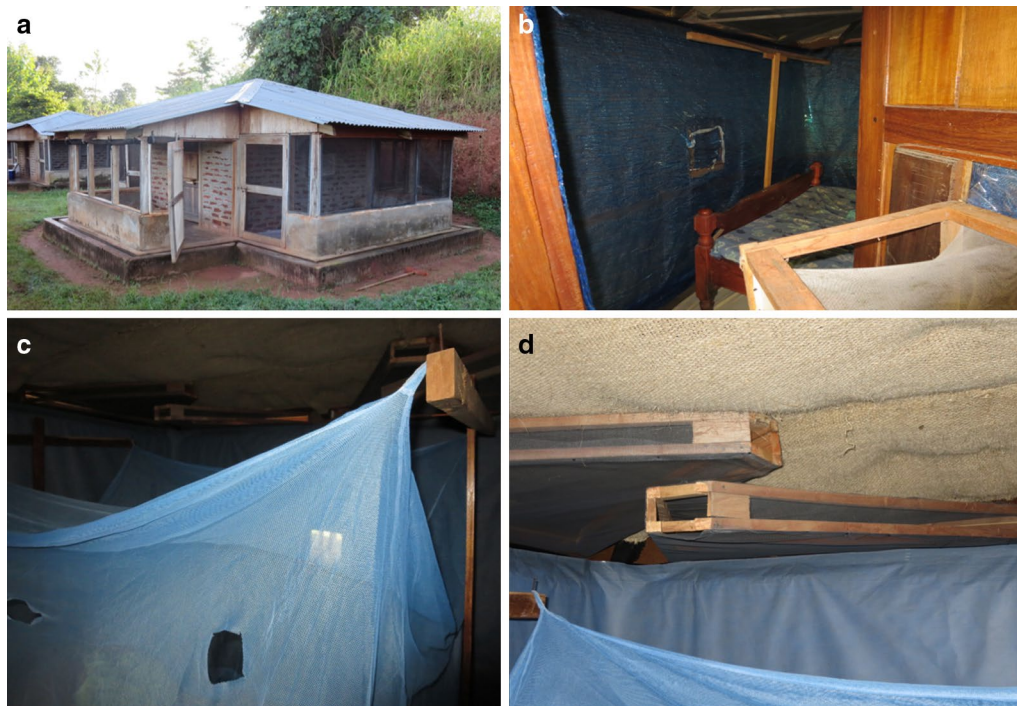
Fig. 1 a East African experimental huts in Zeneti village, Muheza District, northeast Tanzania. b Pyrethroid ITWL (ZeroVector®). c Non-pyrethroid ITWL (PermaNet® Lining) + LLIN (Interceptor®) with eaves partially blocked. d Eave baffles and hessian sack cloth ceiling
