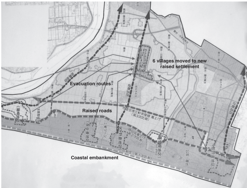
Figure 6. The Iwanuma masterplan: six small settlements concentrated in a new urban centre raised behind three embankments
