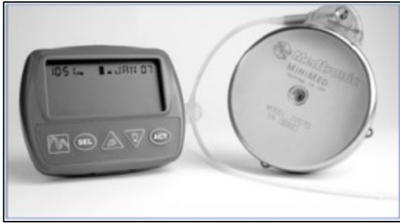
Figure 2. The MIP 2007D implantable pump with hand-held device ( reprinted with permission by Medtronic ).
