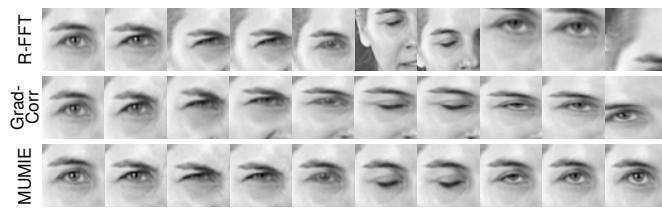
Fig. 10: Registration results for R-FFT, Grad-Corr our method, MUMIE, on a sequence with a disgust expression followed by blinking. MUMIE accumulates little drift error and is not affected by the sudden motions that occur during blinking.
