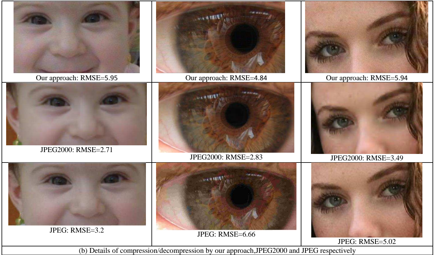
Figure 8: Compressed images by JPEG and JPEG2000 at equivalent compressed file sizes as with our approach.
