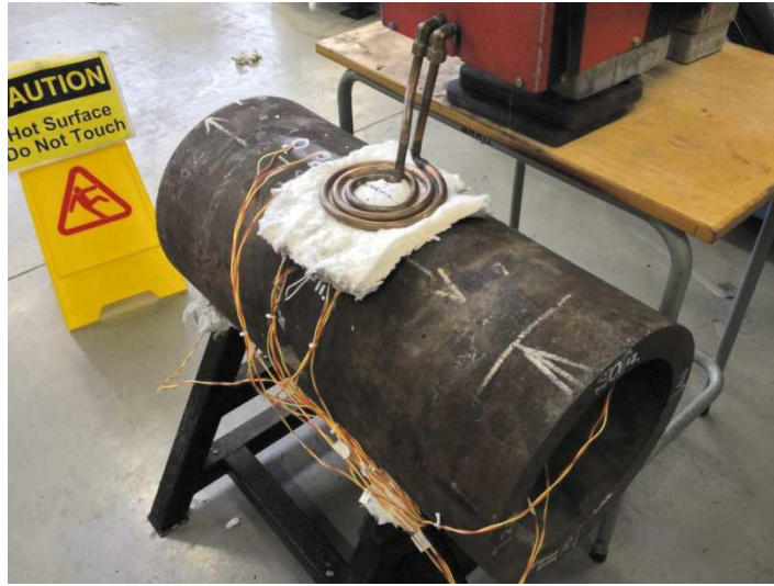
Figure 7. Induction heat treatment of the pipe after completion of the WeldCore® process.
