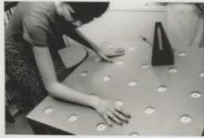
Dunne & Raby - Compass Table The original Compass Table was developed as part of the Kinetic Project. This version is a table made from white wood. Other electronic devices are placed on its surface, the needles, buttons and spin in response to electromagnetic fields produced by the devices.
