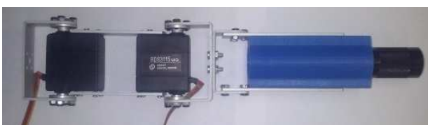
Figure 11. The built robot arm for laser-scanner operations
