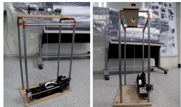
Figure 20. A laboratory prototype of the robotic system with the inkjet printer
