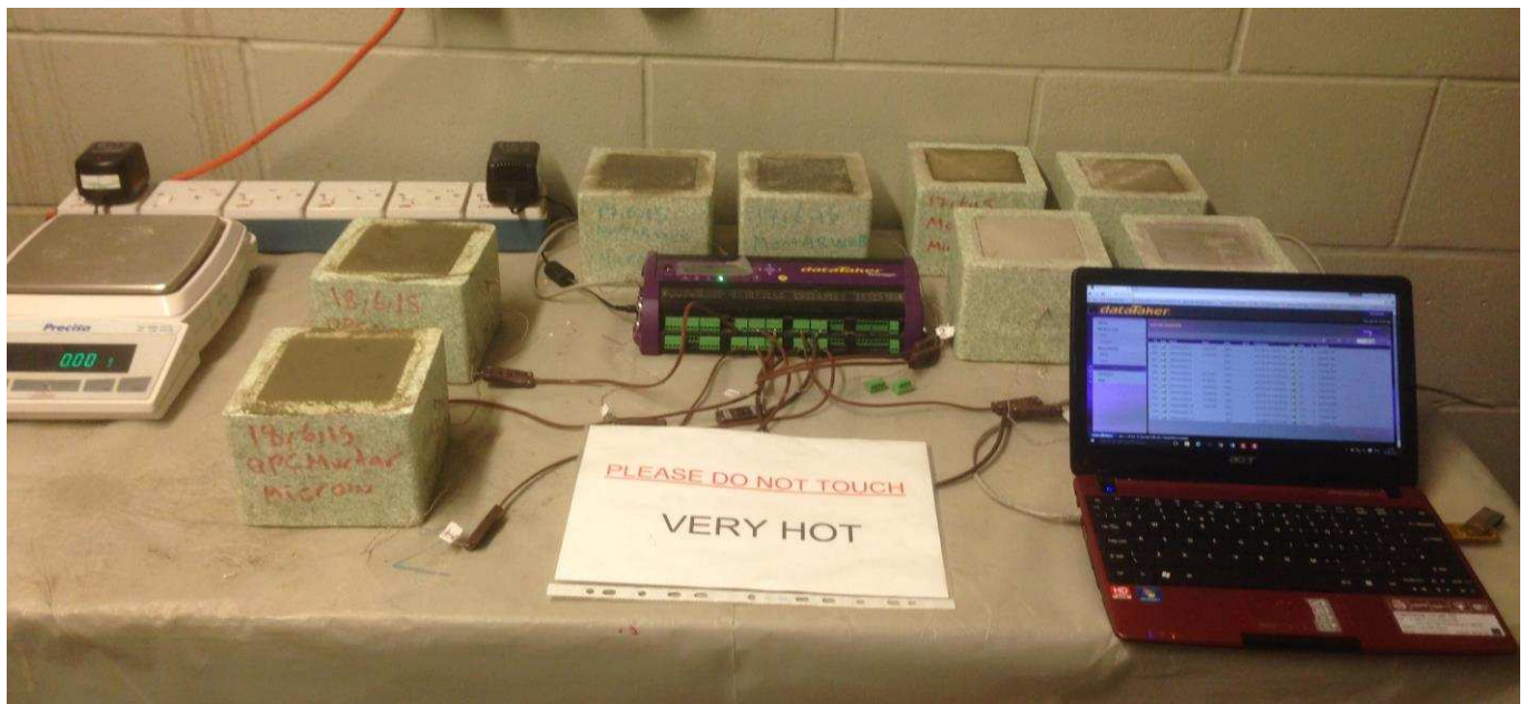
Figure 2. Set up for monitoring internal temperature
