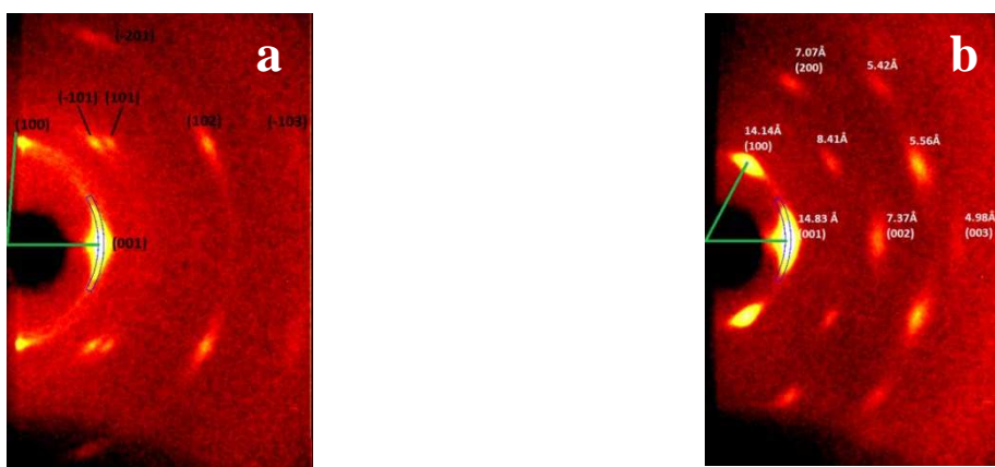
Figure 5. The diffraction patterns of (a) \alpha -PdPc and (b) PdPcF 16 thin films, obtained by 2D GIXD technique.
