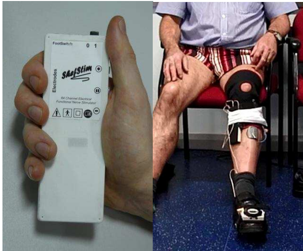
333 334 Figure 5: ShefStim stimulator (left) being used by a subject during setup (right)
