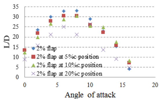
Fig. 10 Lift to drag ratio with Gurney flap mounted at different position as a percentage of the chord.
