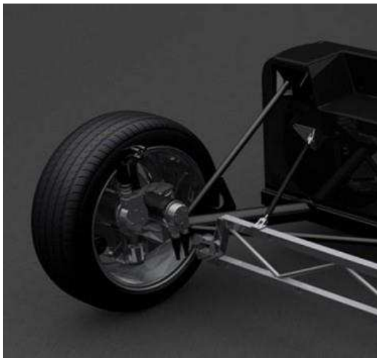
Figure 8. Venturi prototype and link of the Active wheel to the chassis
