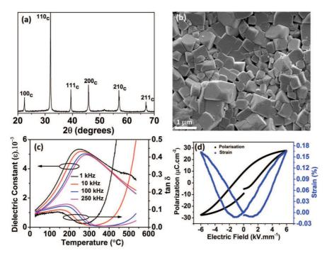
FIG. 1. (a) XRD pattern of KBNFT9 at RT; (b) the ceramic microstructure of KBNFT9; (c) permittivity and tan  $\delta$  versus temperature for KBNFT9 ceramics; (d) P-E and S-E loops for KBNFT9 bulk ceramics at RT and at a frequency of 1 Hz.
