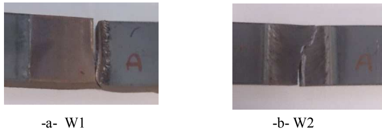
Fig. 15: Fatigue test of a-high speed welding and b-low speed welding.
