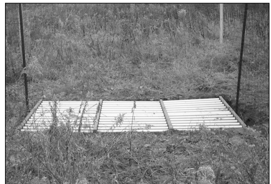
Figure 2. Experimental deer guard installed at a deer enclosure at DeSoto National Wildlife Refuge, Iowa. The guard consisted of 3-roller conveyor panels suspended over a 400-mm-deep cavity. Guard dimensions were 1.5 m × 3 m.
