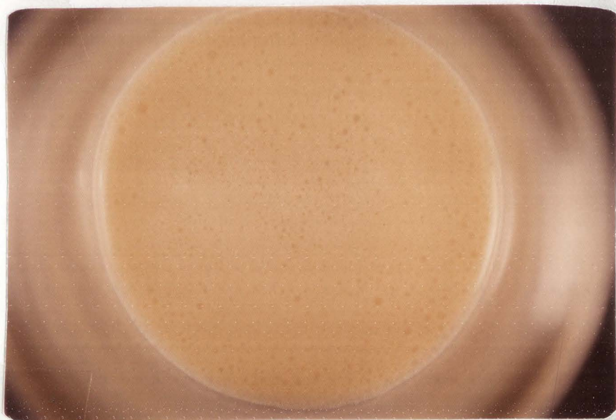
(b) A churned sample after heating to 37.7 C, showing liquified milkfat on the surface.
