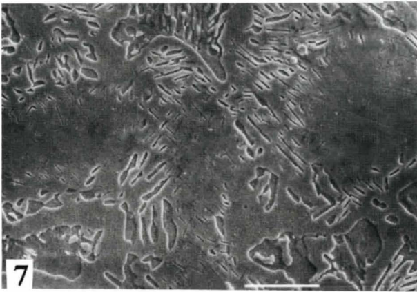
Figure 5. High-magnification photomicrograph of ACBC Spartan Plus. Widmanstätten precipitates in the dendrites and embedded particles in the interdendritic region can be clearly seen. As in Figure 4, the particles may be a secondary phase or the etching pattern of a eutectic constituent. Bar = 1 \mu\text{m} .
