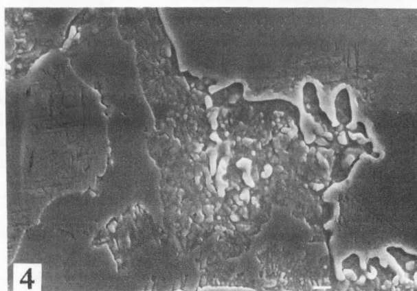
Figure 1. Microstructure of as-cast and bench-cooled (ACBC) Spartan. The dendritic structure is evident. Bar = 100 \mu\text{m} .
