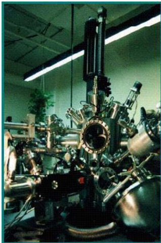
Fig. 1 USU Materials Physics Group UHV electron emission spectroscopy vacuum chamber.
