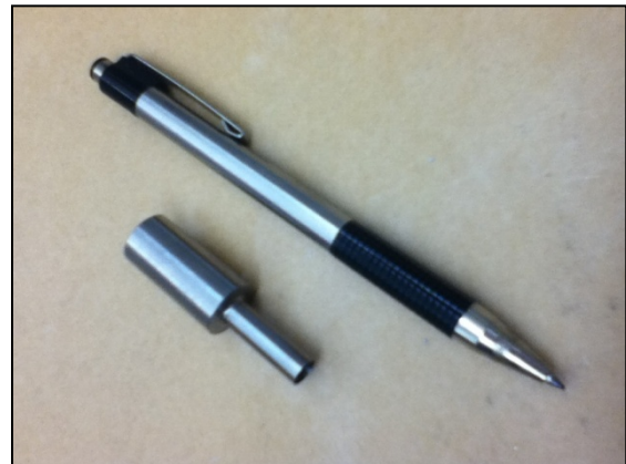
Fig. 2 A Faraday cup currently in use inside the UHV chamber (pen shown for scale).
