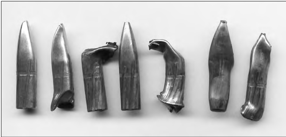
Figure 1: Copper-jacketed compressed, metal powder bullets (140 grain Barnes MPG bullets) after being fired into the head and spinal cord of tuberculosis-infected captive elk ( Cervus elaphus ) at ~1000 fps terminal velocity. While instant incapacitation was achieved, many of the recovered bullets did not break apart, even after striking the ground, because of the low velocity.
