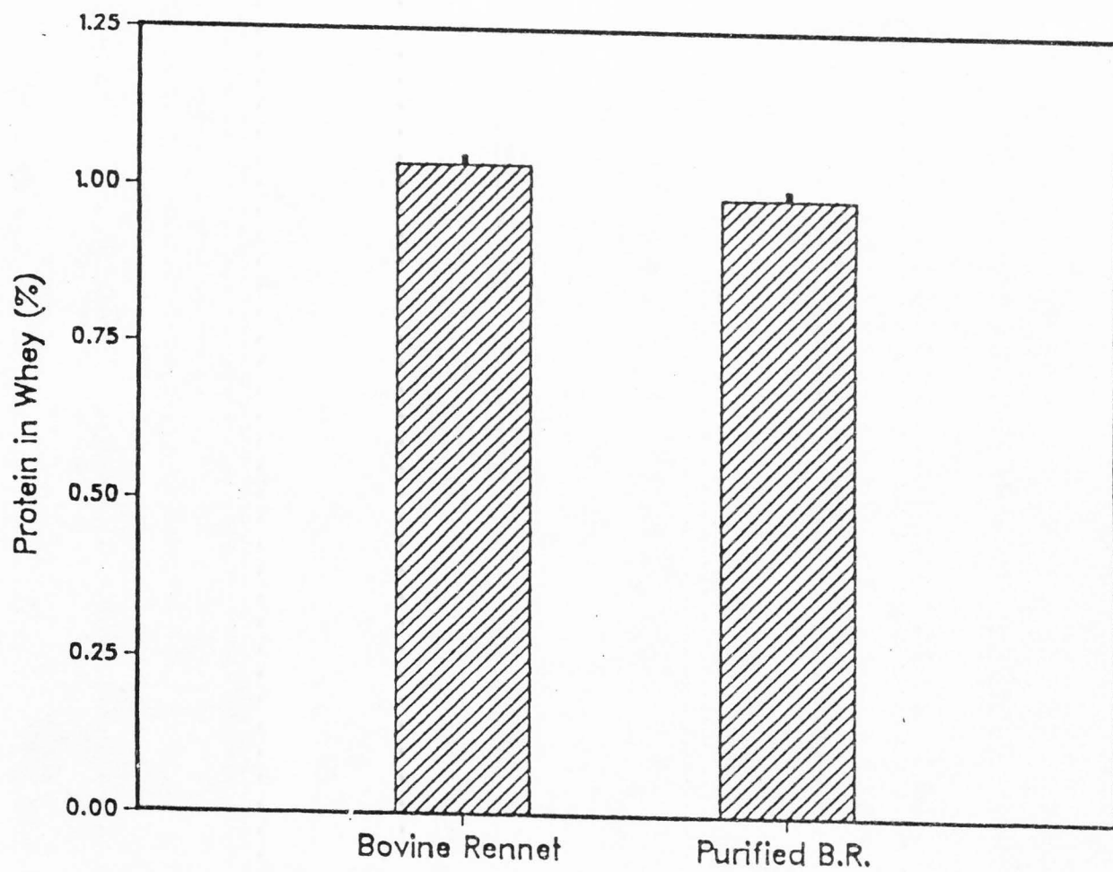
Figure 4. Percent protein lost to whey from commercial and purified bovine rennet. Lines on the top of bars represent standard error of means.
