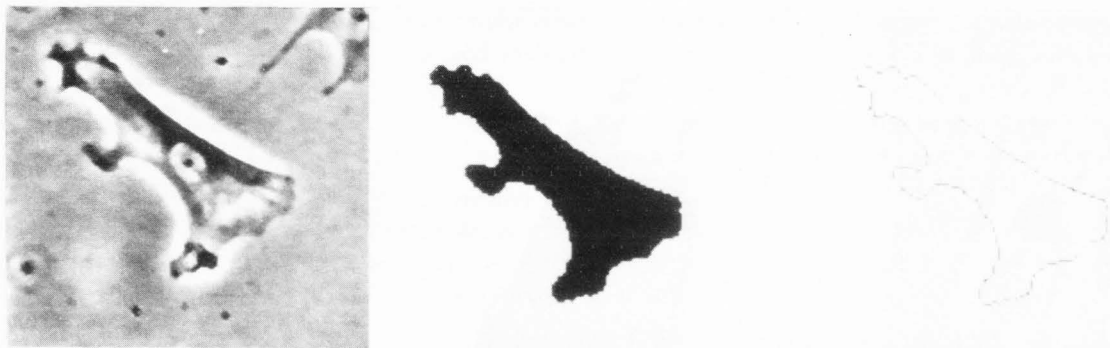
Figure 6. Three digital images captured from the phase contrast microscope of a reasonably spread periosteal cell cultured on tissue culture polystyrene for 2 weeks, showing from left to right the original 256 grey scale image, the cell shape following edge detection with a Sobel filter and the final binary trace of the cell periphery. Field width of each of 3 images: 340 \mu m.
