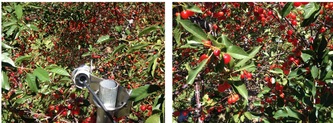
Fig. 4.3.3. 2014 Kaysville tart cherry example IRT field of view. Much fruit, some branches and some ground can be seen in the picture.
