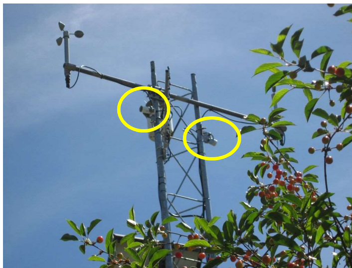
Fig. 4.3.6. Infrared radiometers mounted near the top of a weather station tower. Generally, one sensor faced east and one faced west.
