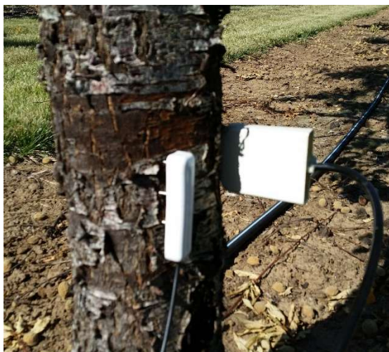
Fig. 3.3.9. GS3 and CS655 installed in a peach tree trunk revealing some exposed waveguide near the sensor head.
