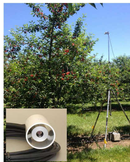
Fig. 4.3.1. Infrared radiometer installed adjacent to a single tart cherry tree.
