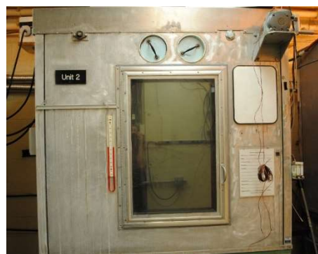
Fig. F.2.1. Partially-retrofitted growth chamber
