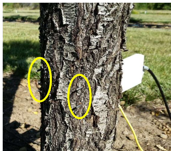
Fig. 3.3.10. CS655 and TDR-315(L) sensors protruding through a peach tree trunk.
