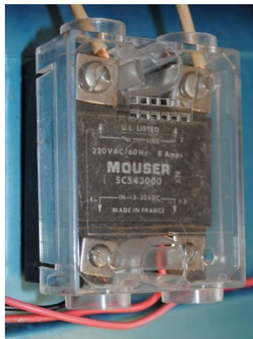
Fig. F.2.4. Solid state relays interfaced datalogger DC signals with 120 V electricity.
