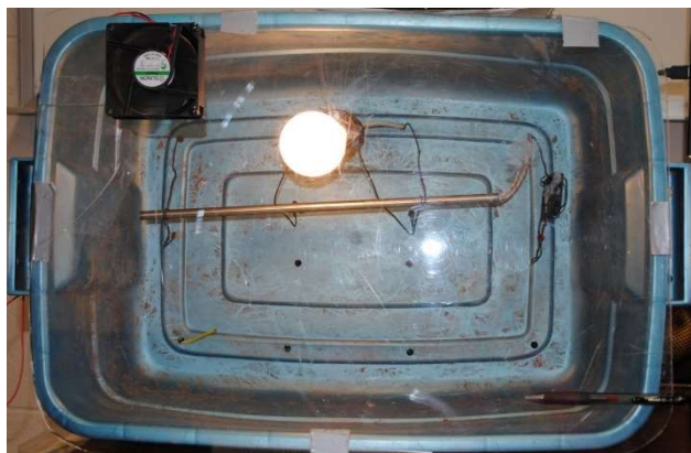
Fig. F.2.5. Simulated growth chamber used to test programs and real-time interfaces.
