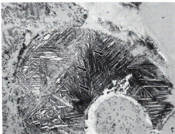
Figure 6. Transmission electron micrograph showing severe degradation of the tricalcium phosphate after 8 weeks of culture. Note the well defined crystallite boundaries (arrows). Field width: 9.4 \mu\text{m} .
