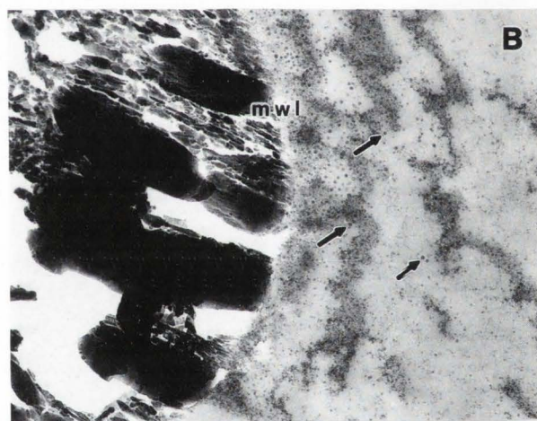
Figure 6. Transmission electron micrograph showing severe degradation of the tricalcium phosphate after 8 weeks of culture. Note the well defined crystallite boundaries (arrows). Field width: 9.4 \mu\text{m} .
