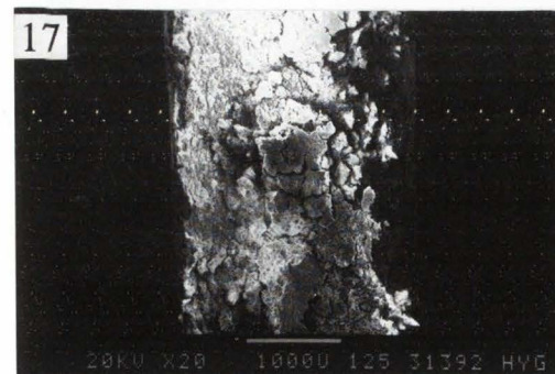
Figure 11. Outer surface of a new catheter (top) at low magnification (bar = 1000 \mu\text{m} ).
