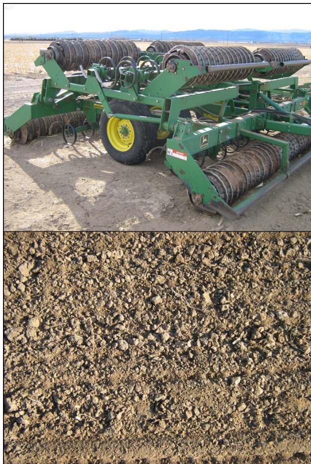
Figure 2. Example of a cultipacker (top) and the firm seedbed (bottom) it can create prior to seeding into cultivated ground. Although a fine, firm seedbed is ideal in most situations, in this example, the soil is high in clay and it is actually good to see the small clods on the surface. If clay soils are worked too fine (i.e., powdery), they will form a hard crust following wetting from rain or irrigation which can impede emergence of birdsfoot trefoil seedlings.
