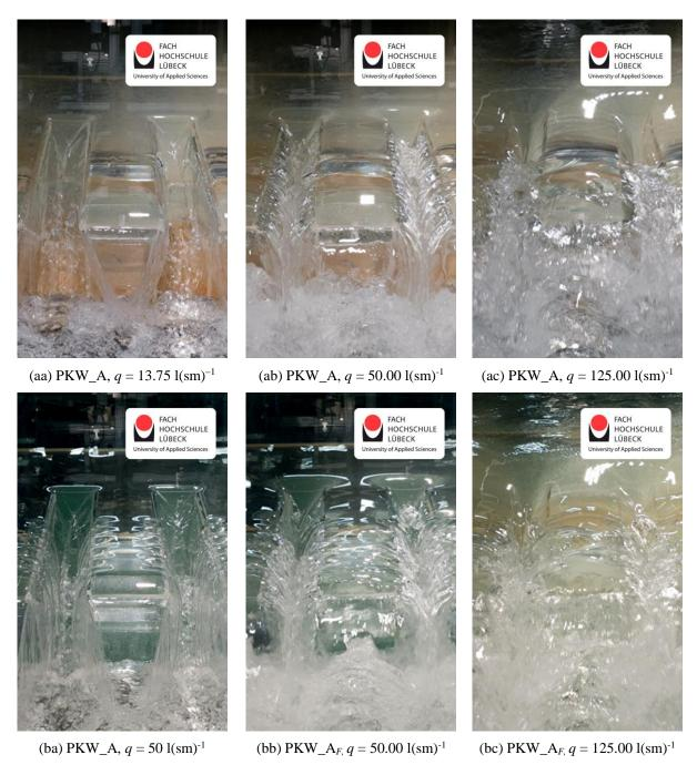
Figure 11. Detail Photograph of the inlet in centerline of the PKW\_A and PKW\_A<sub>F</sub>.
